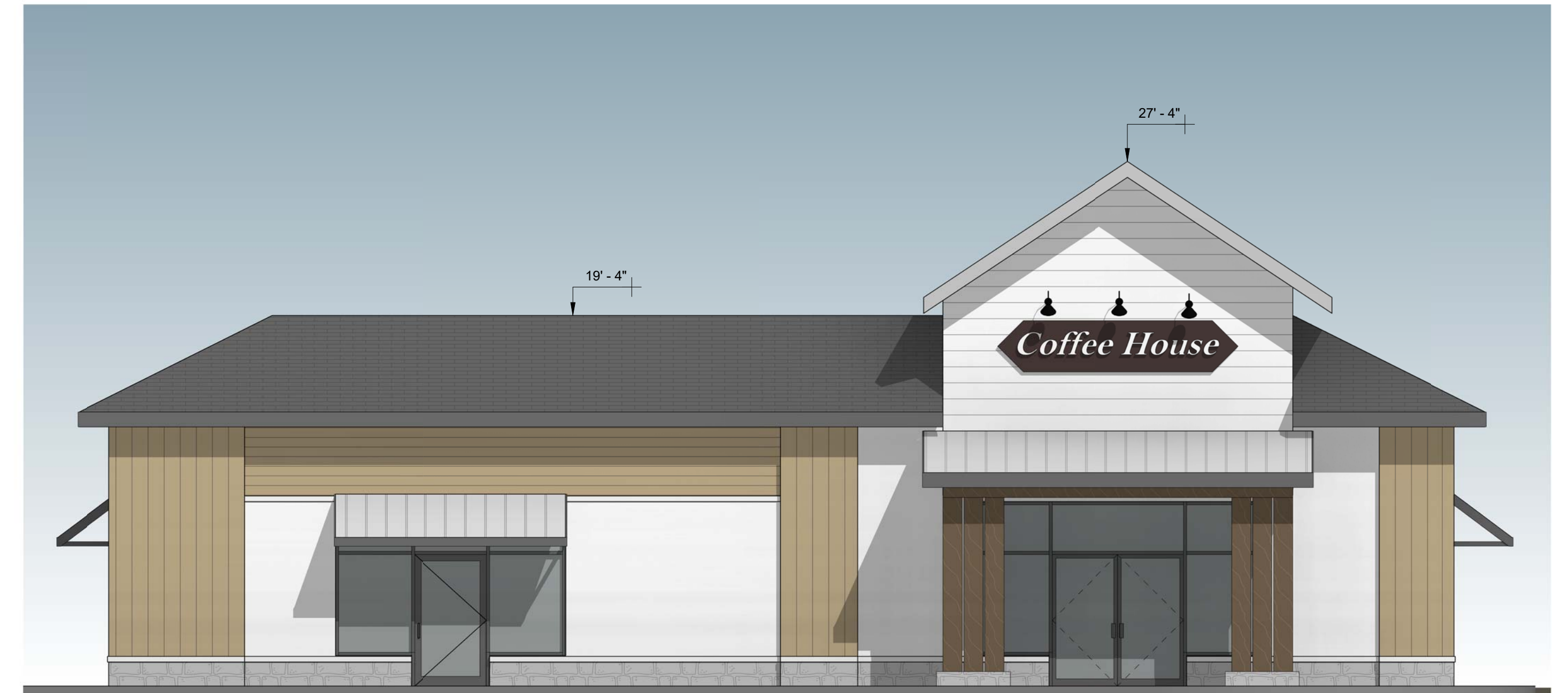
WALL AREA=470 S.F., MAX.SIGN AREA=23.5 S.F. (5%) WALL AREA=650 S.F., MAX.SIGN AREA=32 S.F. (5%) TENANT 13 TENANT 14 ① TENANT 13 AND 14 - WEST ELEVATION 3/16" = 1'-0"
